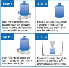
The filter cartridge should be replaced every 6 months or sooner if the flow of water to the dispenser or ice maker decreases. To reset the Filter Change Indicator on the Dispenser Control Panel, simultaneously PRESS and HOLD and D pads until the Filter Change Indicator lamp begins blinking. Release the pads and the lamp turns off.
